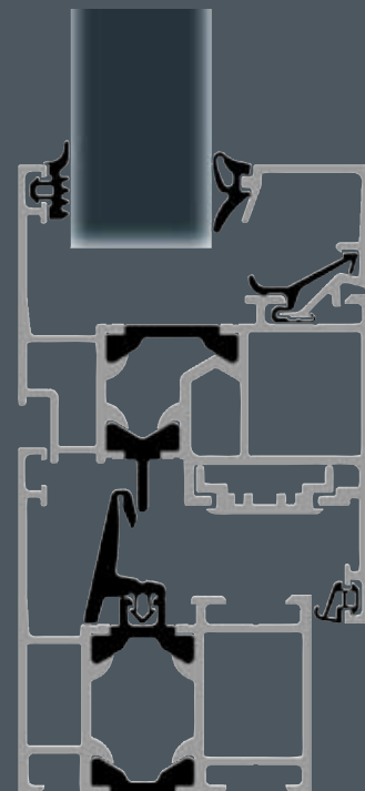
Schüco AWS 50 Thermally insulated frames with centre sealing gasket
