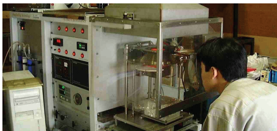
Fig. 2-8 Fire test in Japan, ISO 5660-1
