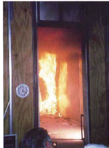
Example of Interior Room Corner Test
